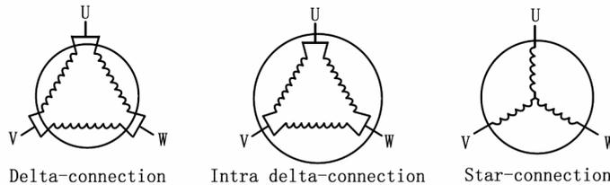
Figure 4: Motor connections
